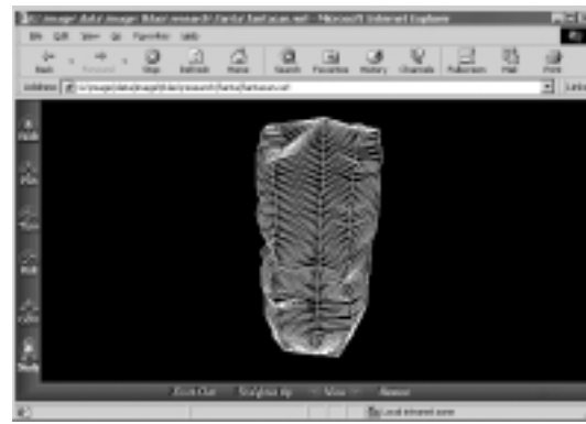
Figure 7 : Wireframe Model of a Deformed Can
