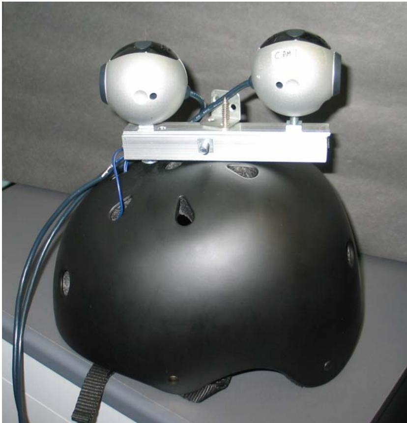
**Figure 1b:** Close-up of the head mount with two cameras
