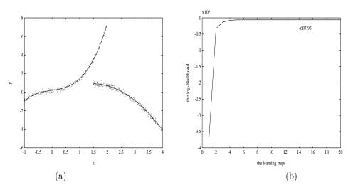
Figure 2: Piecewise 3rd polynomial approximation. (a) 1000 samples from  $y=a_1x^3+a_3x+a_4+\varepsilon, x\in[-1,1.5]$  with prior  $\alpha_1=0.4$  and  $y=a_2'x^2+a_3'x^2+a_4'+\varepsilon, x\in[1,4]$  with prior  $\alpha_2=0.6$ , where x is uniform random variable and z is from Gaussian N(0,0.15). The two curves through the clouds are the estimated models of two expert nets. (b) The evolution of the log-likelihood.
