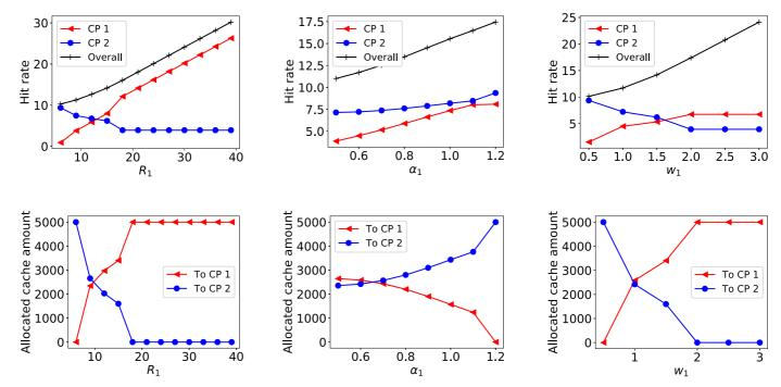
Fig. 6. Effect of the parameters on hit rates and cache resources allocated to content providers.
