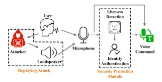
Fig. 1. Classical workflow of the VA system
