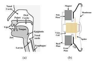
Fig. 2. Structure illustration of two speakers, presenting obvious differences. (a) Human articulator. (b) Electronic loudspeaker.
