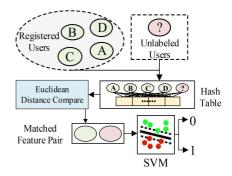
Fig. 10. Structure of the liveness detection model in LiveProbe (features of one phoneme's critical frames as inputting).
