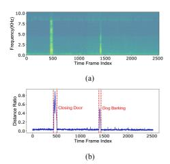
Fig. 6. Background noise patterns from a living room. (a) Spectrum of background noise. (b) Euclidean distance ratio between 1st frame and subsequent ones.
