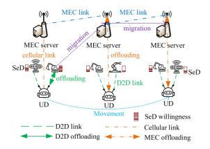
Fig. 1. Industrial task co-offloading in D2D-assisted MEC networks. Computing-intensive industrial tasks are offloaded to MEC servers and SeDs by joint considering SeD willingness and migration cost, targeting minimal system cost, i.e., the sum of task delay and migration cost.
