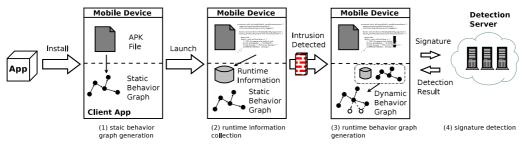
Fig. 2. Overview of MONET. Runtime behavior signature will be generated through static behavior graph generation, runtime information collection and runtime behavior graph generation.
