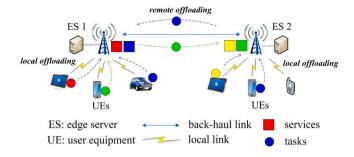
**Fig. 2.** The concept of local edge computing and remote edge computing. At ES 1, the workload marked as red and blue is locally processed, whereas the workload marked green is offloaded to ES2 for remote computation; Likewise, at ES 2 the workload marked yellow is locally processed whereas the workload marked blue is offloaded to ES 1. (For interpretation of the references to color in this figure legend, the reader is referred to the web version of this article.)
