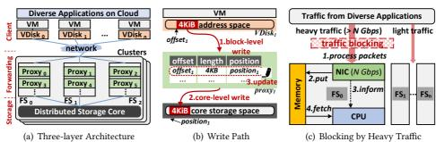
Fig. 1. Illustration on the architecture of a cloud block service and the detailed write path.
