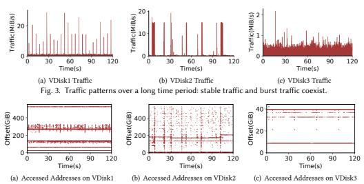
Fig. 4. The distribution of accessed addresses for three typical kinds of VDisks.
