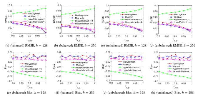
Fig. 2. Estimation error of our method MaxLogHash in comparison with MinHash and HyperMinHash on both balanced and unbalanced set-pairs with k=128.
