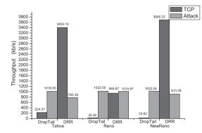
Fig. 10. Result for Low-rate Attack to Single TCP Flow using Tahoe, Reno and New Reno
