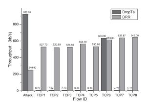
Fig. 14. Result for Single Low-rate Attack to Multiple TCP Flows using New Reno
