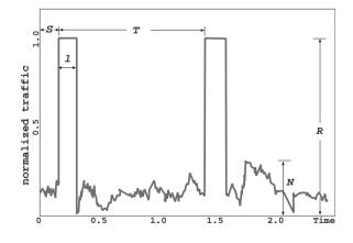
Fig. 1. Low-rate TCP attack traffic with parameters (T, l, R, S, N).
