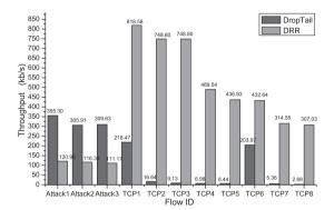
Fig. 16. Result for Synchronized Distribute Low-rate Attack to Multiple TCP Flows using Tahoe
