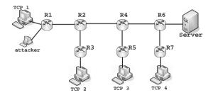
Fig. 19. Network model of Low-rate attack and Multiple TCP flows .
