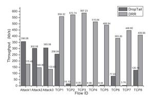
Fig. 17. Result for Synchronized Distribute Low-rate Attack to Multiple TCP Flows using Reno
