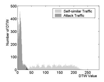
Fig. 8. Probability density functions of DTW values for the attack and the self-similar legitimate traffic.
