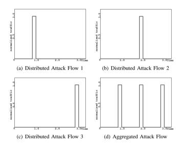
Fig. 3. Distributed low-rate attack with period T=3 and M=3 attack sources.
