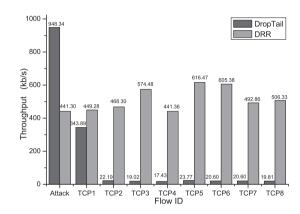
Fig. 13. Result for Single Low-rate Attack to Multiple TCP Flows using Reno
