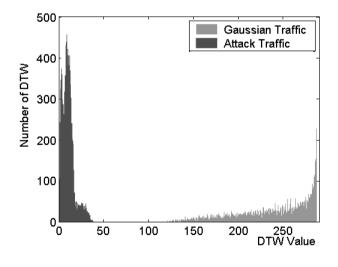
Fig. 7. Probability density functions of DTW values for the attack and the Gaussian legitimate traffic.
