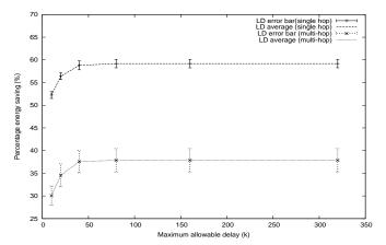
Fig. 6. Percentage energy saving as a function of k for LD heuristic.
