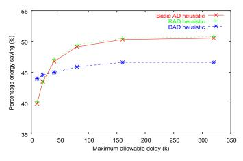
Fig. 5. Percentage energy saving as a function of k for AD, RAD and DAD heuristics.
