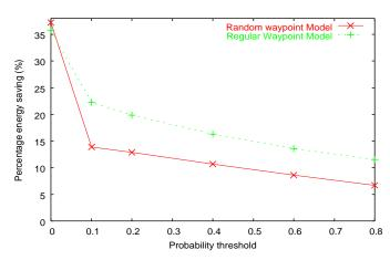
Fig. 1. Percentage energy saving as a function of  $p_{th}$  for MD heuristic.
