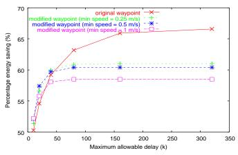
Fig. 10. Percentage energy saving as a function of k for LD heuristics.
