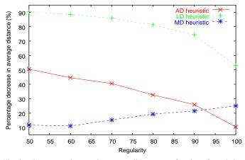
Fig. 8. Percentage decrease in average distance as a function of regularity for MD, AD and LD heuristics.
