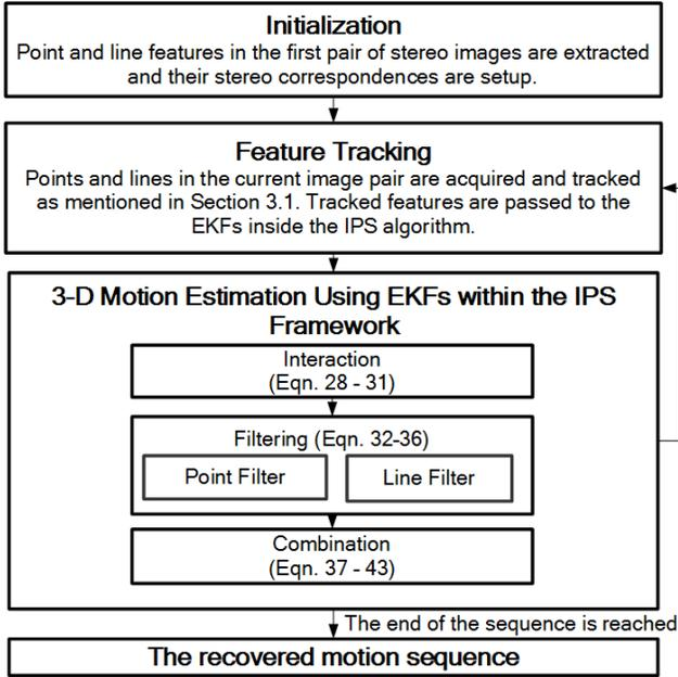
**Fig. 2:** A summary of the proposed 3-D motion tracking method that uses multiple extended Kalman filters within the interacting probabilistic switching framework.
