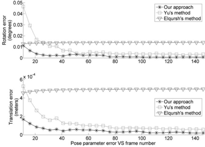
Fig. 7: The mean accumulated rotation (top) and translation (bottom) errors versus frame number of the algorithms under comparison.
