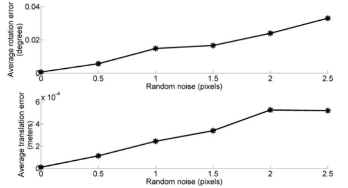
Fig. 5: The accuracy of the recovered poses varies as a function of measurement noise.
