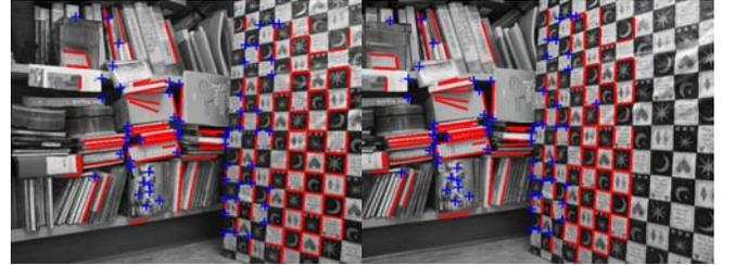
**Fig. 3:** The extracted and matched point and line features in a stereo image.
