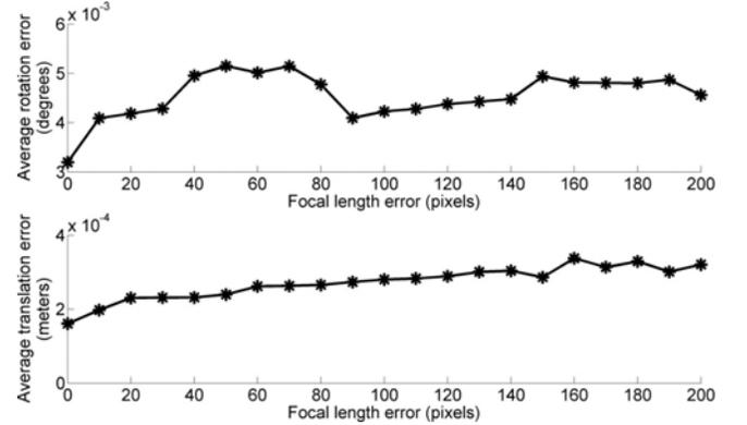
Fig. 6: The accuracy of the recovered poses varies as a function of errors in the calibrated focal length.
