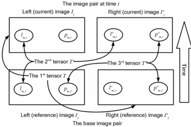
**Fig. 4:** A visual representation of the trifocal tensor arrangement. The first tensor  $T$  involves both points and lines in images  $I_1$ ,  $I'_1$  and  $I_t$ . The second tensor  $T'$  involves only lines  $l_{m,1}$ ,  $l_{m,t}$  and  $l'_{m,t}$ . The third tensor  $T^*$  involves only points  $p_{m,1}$ ,  $p'_{m,1}$  and  $p'_{m,t}$ .
