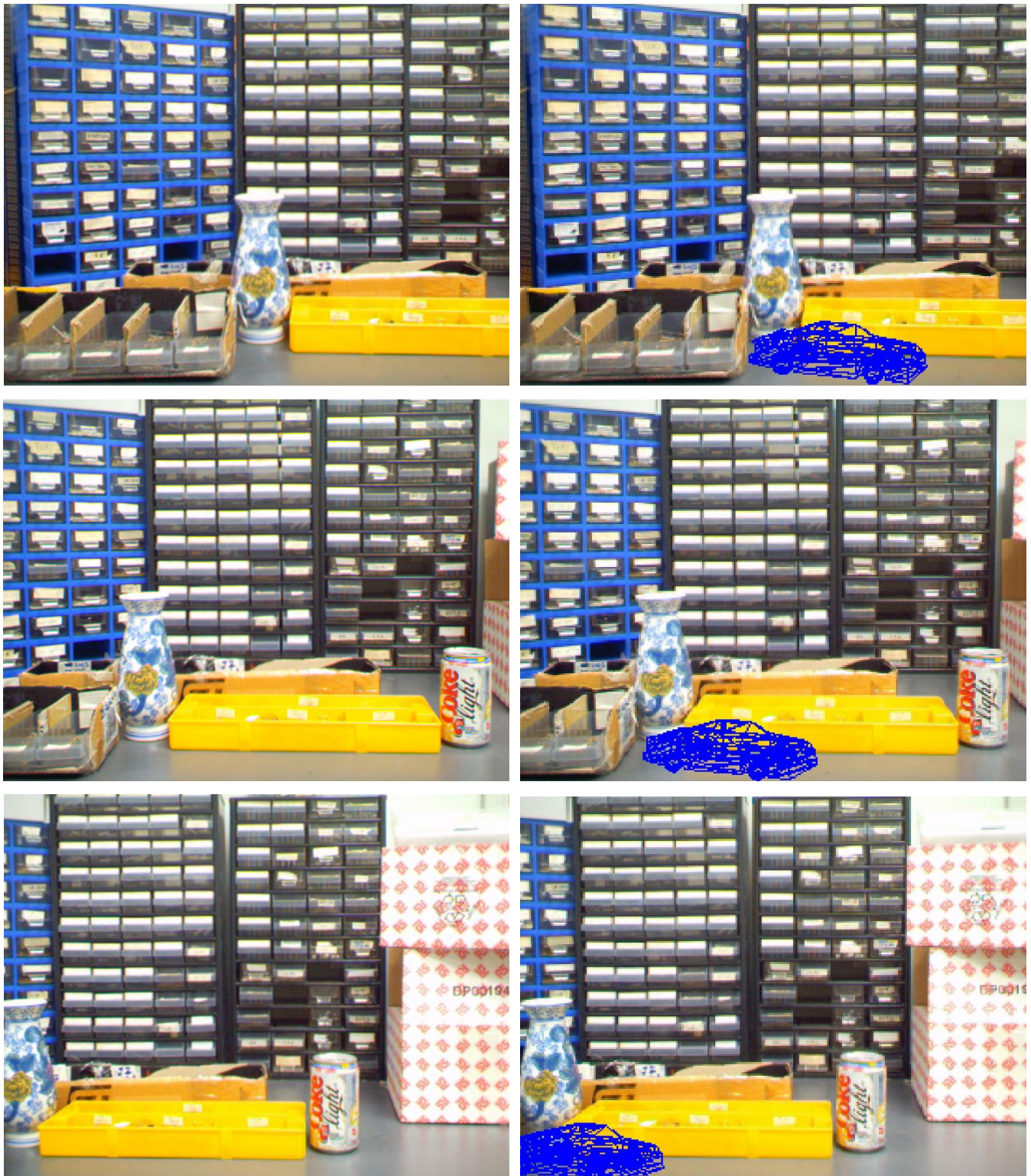
Figure 8. Results of inserting an artificial object into the laboratory scene sequence using the proposed approach. The left column: The 1 st , 50 th and 100 th image of the sequence. The right column: A synthetic car, which is drawn by wire-frames, was augmented into the scene.
