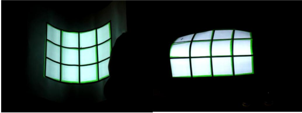
Figure 11. The green grid is projected while the black grid is printed. The coincidence of the green grid with the black grid indicates the projection accuracy of the system.
