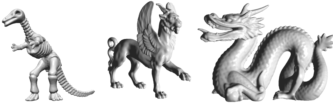
Figure 5. Examples of large-scale implicit surface modelling. The Dino (56K points, 2.8s) with complex edge structures is modelled by 43K bases, and the Caltech feline (200K points, 11.5s) is modelled by 100K bases. The Stanford dragon contains more than 400K data points.
