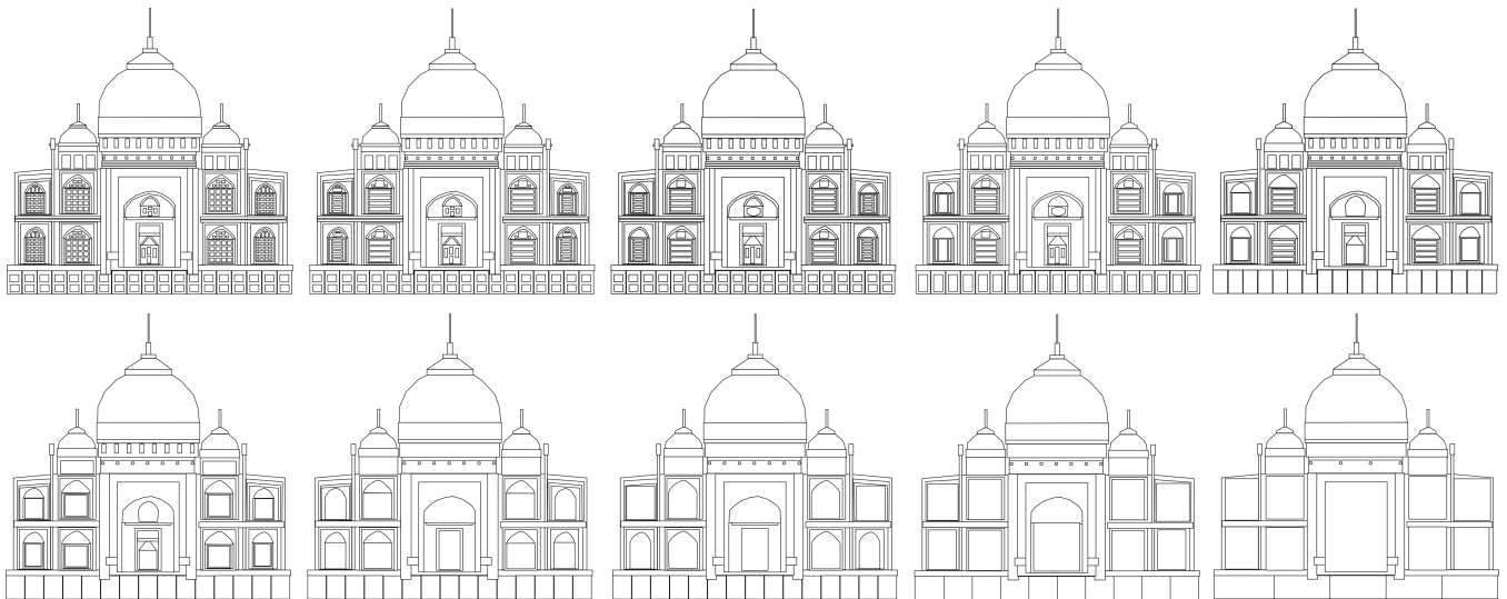
Figure 3: Clean rendering of Figure 14 in the paper (from left to right, top to bottom row). Four out of six small elements in the original inner window (upper part) are replaced by an embracing square. The remaining two elements are removed using the level of detail threshold t_{LOD} . The horizontal regular pattern below the central dome is grouped by regularity and simplified by summarization.
