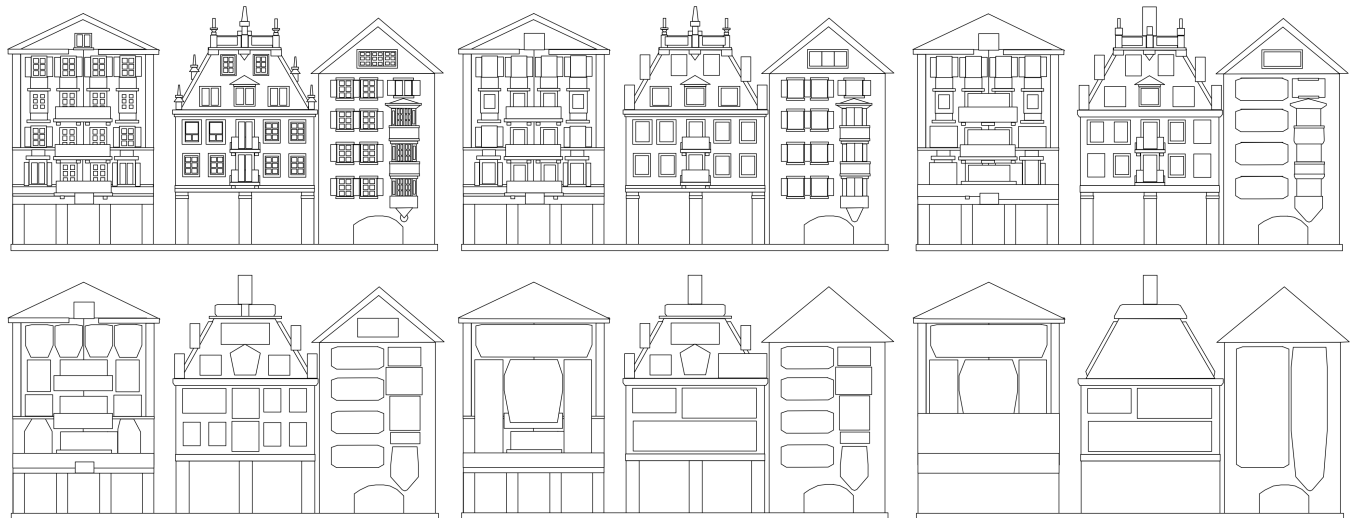
Figure 9: Six simplification iterations of a complex building (from left to right, top to bottom row).
