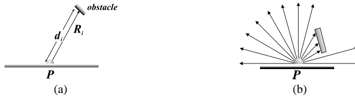
Fig. 2. (a): Ray R_i intersects with an obstacle. (b): n evenly distributed rays emitted from point P .
