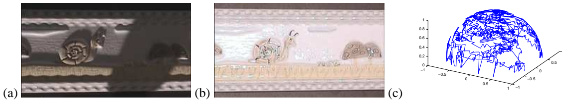
Fig. 1. Two typical noisy photometric images for Snail captured by our simple system. (a) is significantly contaminated by shadows, and (b) is corrupted by highlight. (c) A typical trajectory of the estimated light directions shows that they are scattered and very noisy.
